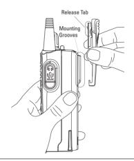
To attach, align mounting rails of the belt clip with the grooves of the radio.
